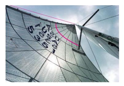
**OPTIMUM SAG**: A looser headstay helps create a more powerful genoa shape with a deeper entry, a farther forward maximum draft, and a flatter trailing edge. This creates a powerful shape that provides both maximum height and speed in underpowered conditions.
