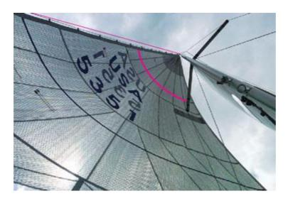
**NOT ENOUGH SAG:** In light winds on a J/24—these photos were taken in 6 to 8 knots—headstay sag is crucial for developing power in the genoa, which in turn generates pointing ability. This sail, set on a tighter headstay, has less depth, and the position of the maximum draft is further aft on the sail. A boat with a sail set this way will likely struggle to keep pace upwind in light air.
