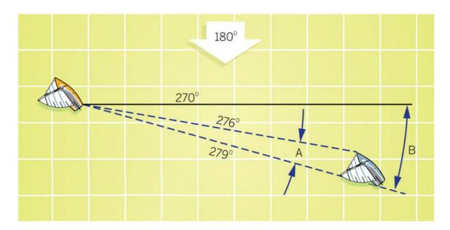
Dividing the difference between bearings for the crosswind and position lines (B) by your opponent's boat length in degrees (A) will provide your lead (or deficit) in boat lengths. In this example: 279-270/3 = 3 boat lengths.
